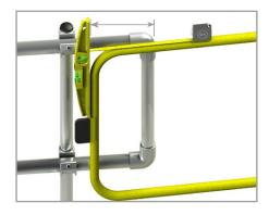
**3.** Measure distance from edge of gate to guardrail upright, and record distance to cut.
